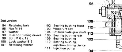
The modified injection timing device and the modified bearing bushing (109) must not be used with the intermediate gear shaft as per the 1st version, because no oil would be able to reach the bearings. In contrast, the modified intermediate gear shaft may be used with the injection timing device and the bearing bushing as per the 1st version.
