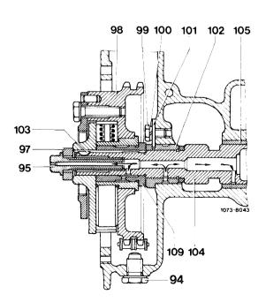
The double diaphragm vacuum pump can be used only with the modified injection timing device (without cam) and with the hollow bolt (95).
