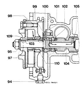
Nut (95) has been modified from poly-stop to a normal hexagon type.
