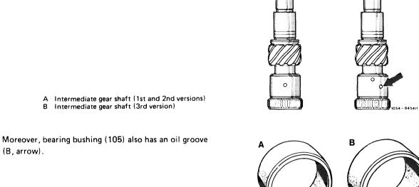
A Rear bearing bushing (1st and 2nd versions) B Rear bearing bushing (3rd version)
